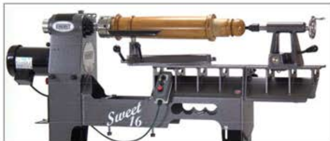
Positioned the gap at the end of the bed to turn long spindles. Note banjo bridges gap.
