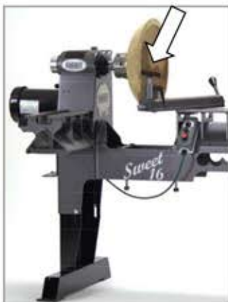
Above: Move the gap section to the headstock and turn up to 32" diameter. Move the tool rest to either side of the work.
