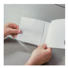
It is important that you cut out the two black semicircles so that you have notches in your paper. Open the folded paper and insert the filter material so it is at the far edge of the filter holder.
