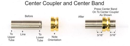
• Next, press the lower tube (shorter tube) onto the short end of the center coupler assembly as shown below.
