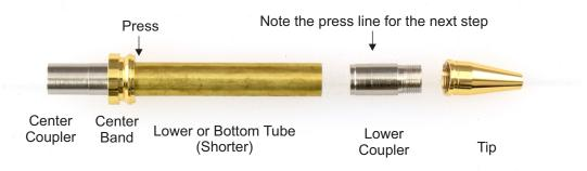
• Press the lower coupler on to the lower end of the lower tube (shorter tube) as shown below. Press the lower tube up to the line in the lower coupler and stop. This is critical.
